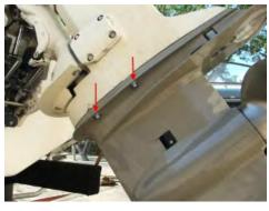
1.7 (Above) Using a 9/16 socket, remove the four mounting bolts (red arrows). There are two on each side. These are the last bolts holding the gearcase to the midsection. The unit will be able to drop when they are removed, so be prepared.
