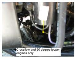
1.2 (Above) Remove the cowling from the engine. If your engine is a cross flow or 90 degree looper, remove the bolt that se-cures the shift rod to the shift linkage (yellow arrow). It is located below the carburetors. On some models, it is much easy to access the bolt if you remove the lower cowlings. If your engine is a 60 deg (non E-TEC) the procedure is different, see below.
