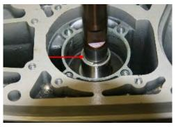
Forcefully push the upper driveshaft down into the lower driveshaft. Then pull back up. The driveshaft should the end of the upper driveshaft. Use the screwdriver and remove it. Discard the two wire clips. They will not be reused in the SEI unit.
