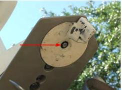
**1.5** (Above) Remove the trim tab bolt with a 7/16"socket (red arrow). Note the angle of the tab so that you can duplicate it on the SE306 unit.
