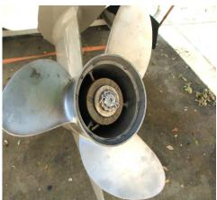
1.1 (Above) Remove the cotter pin for the prop nut. Slide off the castle nut cover. Block the propeller with a piece of wood to keep it from spinning while you loosen and remove the prop nut. Remove the propeller and thrust washer. The thrust washer may stick in the propeller.
