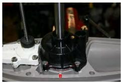
2.10 (Above) Slide the water pump housing as assembled down the driveshaft. Align the wedge held with the o'ring with the corresponding slot in the impeller and slide the housing down until it contacts the wear plate. The impeller will push the o'ring off of the key and the o'ring will settle into the groove at the bottom of the impeller. Using a 7/16"socket, install the four provided screws (A) and tighten evenly to 60 to 84 in. lbs.
