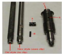
The picture above shows the 1989 through 1992 and 1993 and newer upper drive shafts. The lower drive shaft (D), clip (A), and roll pin (B) are also shown.
