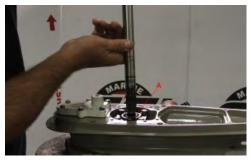
2.2 (Above) Installation of the upper simple and straight forward. Simply in the upper driveshaft carrier (A) and align the splines with the lower shaft. The upper shaft will drop down until it contacts the retaining clip in the lower drive shaft. Softly hit the end of the upper drive shaft with a mallet or block of wood until you feel it engage the teeth of the clip. You will know that the shaft is installed properly when you can no longer pull the upper drive shaft back out.
