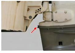
1.4 (Above) Some models use a pitot pickup in the lower unit for the speed-ometer. If your unit is so equipped, disconnect the tube before removing the unit. The unit pictured does not utilize the pick-up. The arrow points to the nipple where it would be hooked up.
