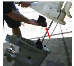
**3.1** (Above) Most units will have a lower exhaust extension (arrow). It may stay stuck in the midsection when the lower unit was removed. Remove it and inspect the seals on both ends. Replace as necessary. Before installing the SEI gearcase, push the extension piece back into place. The upper seal should hold it in place. Slide the propeller onto the propshaft. Do not install the nut at this time.
