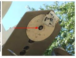
**3.5** (Above) Re-install the trim tab. Tighten the mounting bolt to 35-40ft.lb.
