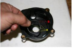
2.8 (Above) An o'ring must be installed in a groove in the plastic housing before the liner can be installed. Place a small dab of adhesive in the areas marked (A). Place the o'ring (B) in the slot.
