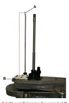
2.4 (Above) Determine the correct shift shaft height for your specific model in a service manual. The measurement is from the centerline of the hole at the top of the shaft (A) to the mounting surface of the gearcase (B). Thread the shift shaft in or out until the measurement is reached. The bend at the top of the shift shaft will face the front of the gearcase.
