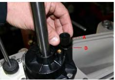
**2.11** (Above) Insert the grommet (A) into the water outlet (B) of the housing. Install the grommet with the inside taper facing up.
