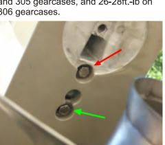
**3.4** (Above) Install the 3/8"bolt (red arrow) and tighten to 22-24ft.-lb on 304 and 305 gearcases, and 26-28ft.-lb on 306 gear cases. Install the 7/16"bolt (green arrow) and tighten to 30-32 ft.lb for 304 and 305 gearcases, and 45-50ft.lb on 306 gearcases.
