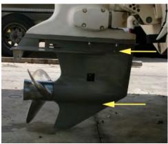
**3.10** (Above) Remove the drain and fill plugs (arrows). Thread a gear lube pump into the threads of the drain plug lower plug). Pump gear lube slowly into the gearcase until it comes out of the vent plug (upper plug). Re-install the vent plug, then quickly remove the pump and re-install the drain plug.
