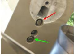
**1.6** (Above) Once the trim tab is out of the way you can gain access to the rear mounting bolt (red arrow). Using a 1/2"socket remove the bolt. Using a 9/16"socket, remove the other rear mounting bolt (green arrow).
