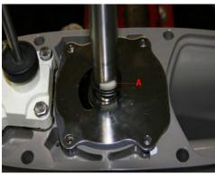
**2.7** (Above) Place the wedge (A) in the slot of the driveshaft. Use the o'ring from the kit to hold the key against the shaft. Make sure the wedge is positioned as pictured.
