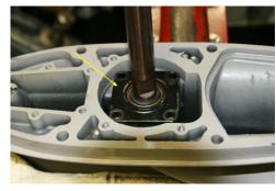
Once it is removed, you will see the upper wire clip (see pic below, red arrow). Use a flat blade screwdriver and slide it off.
