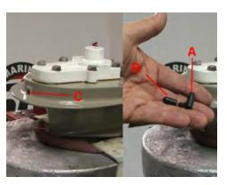
2.13 (Above) Some OMC models had a pitot for the speedometer built into the case. The SEI 305 and 306 have this feature. The elbow (A) and cover (B) are packaged in a small plastic bag with the unit for shipping and need to be installed when you are ready to mount the gearcase. Simply drive the nipple into the hole (C) with the barb facing up. Place the cap over the end of the nipple if you choose not to use the pitot.
