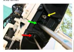
**3.2** (Above) Push the shift shaft on the gearcase down, which puts it into reverse. If you turn the propeller, the driveshaft will now turn also. Insert the ends of the shift shaft (red arrow) and driveshaft (green arrow) into their corresponding holes and lift the gearcase into place. The yellow arrow points to the water tube which you will align with the outlet of the gearcase's water pump.
