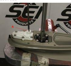
2.3 (Above) Remove the shift shaft from your old gearcase. It simply unscrews and slides out. Apply some grease to the threads to ease installation. There is an o'ring in the hole of the shift shaft cover (A). Thread the shift shaft through the o'ring so that it is not damaged. Some 25 and 30 inch models use a plastic spacer (not shown) which sits on top of the shift cover housing and spaces out a
