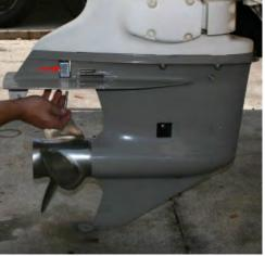
3.9 (Above) Remove the anode from your old lower unit if you are planning on reusing it. Hold the anode (red arrow) in the mounting space and thread the bolt though the case and into the anode. 304 and 306 units use a 5/16" bolt with ½" hex head, which passes through the anode and threads into the gearcase. 305 units use a 3/8" bolt with a 9/16" hex head, which threads into the anode.
