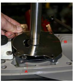
2.6 (Above) Apply aviation gasket sealant to both sides of the base gasket (A) and place it on the gearcase, aligning the holes in the gasket with the bolt holes in the gearcase. Place the wear plate (B) on top of the gasket and align the bolt holes.
