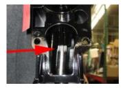
2.4 The next thing to line up is the vertical shaft. It may be necessary to rotate the u-joint assembly clockwise to get the splines aligned. The units should drop completely onto the alignment pins. It may be necessary to push it together to get the water tube into the o-rings.
