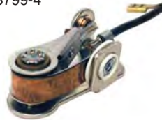
BOSCH 4-Cyl. (Volvo Engines)
