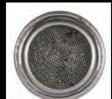
The oil pick-up tube screen is virtually free of sludge.
